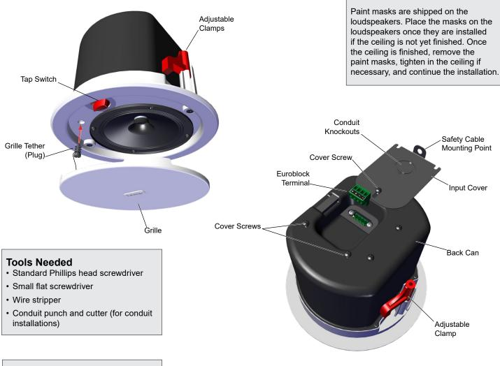
**NOTE:** The installer is responsible for sourcing the proper safety cable to meet all applicable local building codes and standards.
