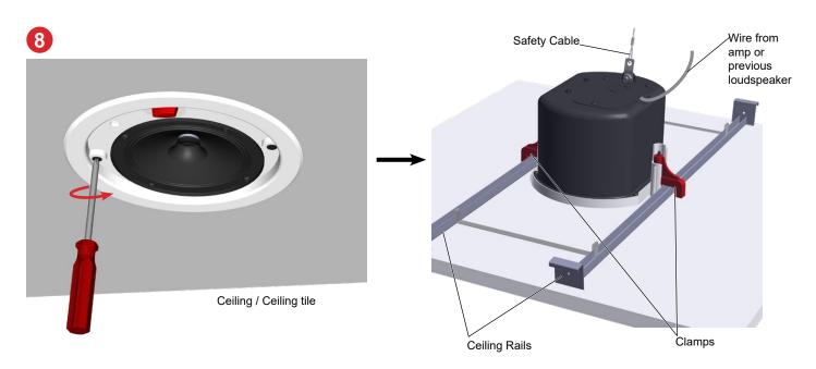
**IMPORTANT:** For closed ceiling applications all connections (wiring and safety cable) must be made with the input cover installed before inserting the unit in the ceiling.
