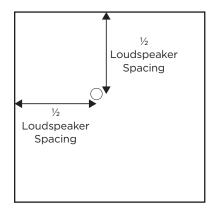
C. The remaining loudspeakers are arranged on a square grid pattern using the LSD. If a loudspeaker would be placed on or beyond the perimeter of the room, delete that row/column of loudspeakers.
