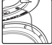
11. Attach grille & bezel seismic restraint to baffle with provided screw.
