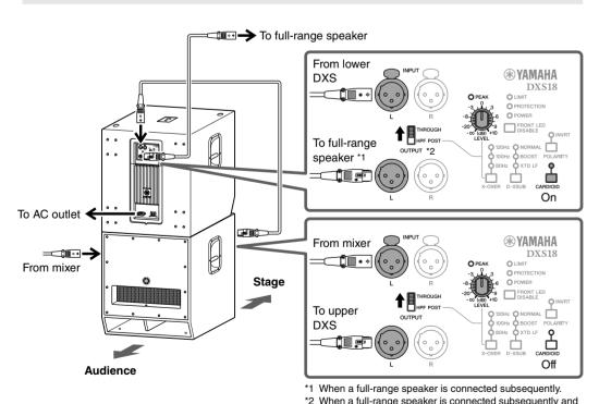
the high pass filter in the full-range speaker is not used, set this to [HPF POST].
