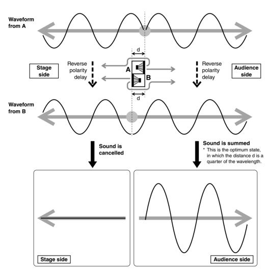
The sound of each speaker is cancelled on the stage side and summed together on the audience side. The directional characteristics of this combination are represented in the polar pattern illustration at right. Since the form resembles a heart shape, it is called Cardioid mode.
