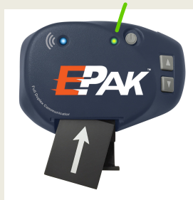
Slide open battery door Arrow/ contacts first
