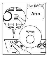
By default, the ioStation 24c is in Studio One operation mode. To switch to Live operation, press and hold the NEXT button while powering on your ioStation 24c, then press the Arm button to enable Live (MCU) operation.
