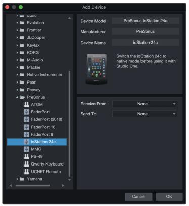
In the Receive From and Send To drop-down menus, select "ioStation 24c."
