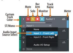
**Note:** Instrument tracks are nearly identical to audio tracks. The Input Source list for Instrument tracks lists available external MIDI devices as well as any virtual instruments that have been added to the Song.
