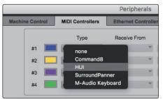
3. Set the Receive From and Send To menus to "ioStation 24c" and #Ch's to 8.
