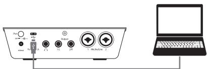
Once you have connected your ioStation 24c to your computer, launch Logic. The ioStation 24c will auto-configure as a Mackie Control Universal device. If for some reason this does not happen, you will need to enable it manually.
