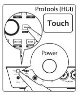
By default, the ioStation 24c is in Studio One operation mode. To switch to Pro Tools operation, press and hold the NEXT button while powering on your ioStation 24c, then press the Touch button to enable Pro Tools (HUI) operation.
