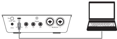
Once you have connected your ioStation 24c to your computer, launch Live to set up the ioStation 24c as a Mackie Control Universal device.
