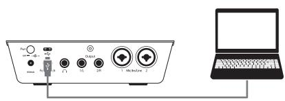
Once you have connected your ioStation 24c to your computer, launch Pro Tools to set up the ioStation 24c as a HUI device.
