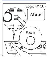
By default, the ioStation 24c is in Studio One operation mode. To switch to Logic operation, press and hold the NEXT button while powering on your ioStation 24c, then press the Mute button to enable Logic (MCU) operation.
