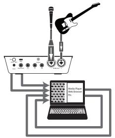
**Power User Tip:** When using either option, you will need to select Outputs 1 and 2 in the audio application you want to record. Make sure to select Outputs 3 and 4 in the audio application in which you're recording to avoid a feedback loop.
