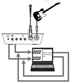
When Loopback is enabled and "Dedicated Loopback Inputs" is selected, the audio from another application will be recorded on the last pair of driver inputs (3/4).
