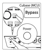
By default, the ioStation 24c is in Studio One operation mode. To switch to Cubase / Nuendo operation, press and hold the NEXT button while powering on your ioStation 24c, then press the Bypass button to enable Cubase / Nuendo (MCU) operation.
