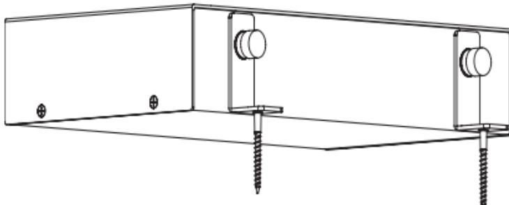
The brackets can be positioned facing in or out as shown to best allow for different types of installations.
