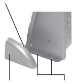
Side cover Holes for screw fastening
