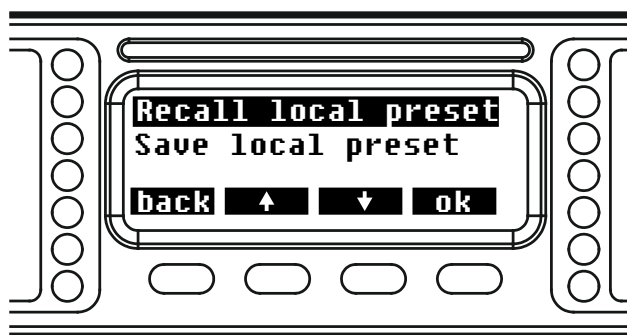
APPENDIX FIGURE 3: The main SmartCard menu is visible when the card is inserted in the amplifier's frontal slot
