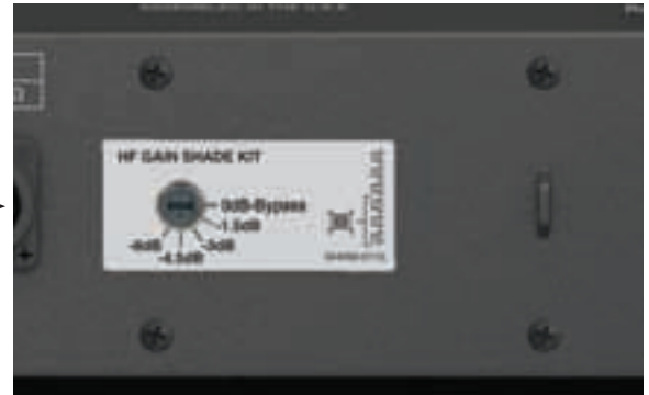
Figure 2. Installed RMSHADE Kit
