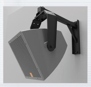
The SAS-200-24 is an efficient, load rated universal wall arm system for mounting objects, such as loudspeakers weighing up to 200 lb/91 kg to walls & other vertical structures. Loudspeaker can easily be attached and aimed from walls and other vertical structures by way of the U-bracket or Yoke with ease of installation and flexibility in adjustment.
