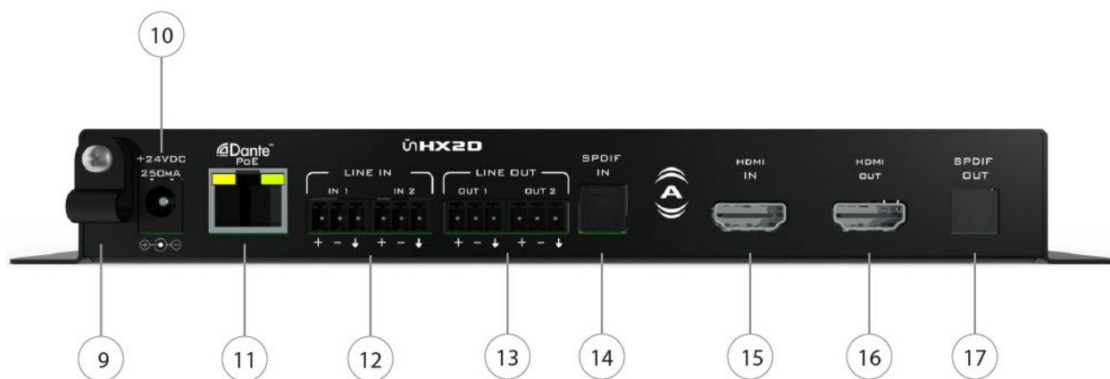
Figure 4 - unHX2D Rear Panel
