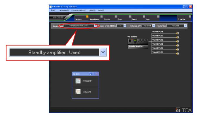
Setting this to "BGM/Paging System" allows connection of a VP-2000 series amplifier to each VM-3000VA and VM-3000E in order to configure simultaneous 2-channel broadcast system for BGM and paging announcement.
