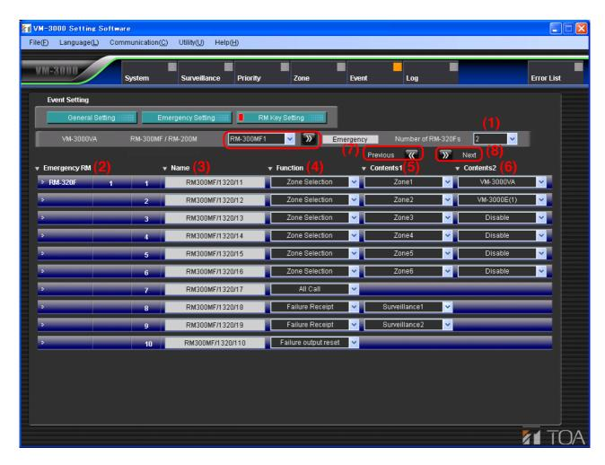
Click the "RM-300MF/RM-200M" selection box or double-arrow button to select the RM-300MF or RM-200M. The display switches to the screen for setting the selected device.
