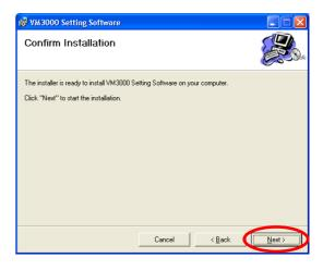
Step 4. Click the Next button to start installing the software.
