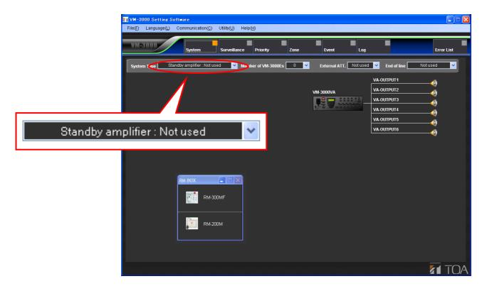
Setting this to "Standby amplifier: Used" sets the configuration to a system that does use a standby amplifier. In such cases, use a VP-2000 series amplifier as the VM-3000VA's standby amplifier.
