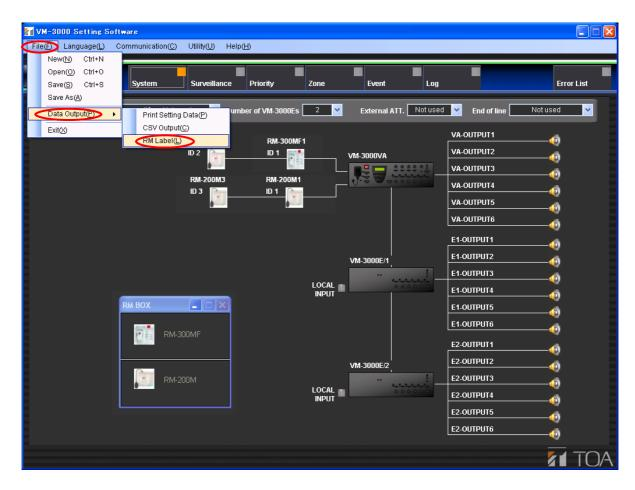
The print preview for the printed labels of all connected remote microphones is displayed.
