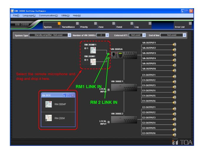
Clicking the set remote microphone icon transfers the display to the RM Key Setting screen (page 53) in Event Settings, allowing the functions of the remote microphone keys to be set.
