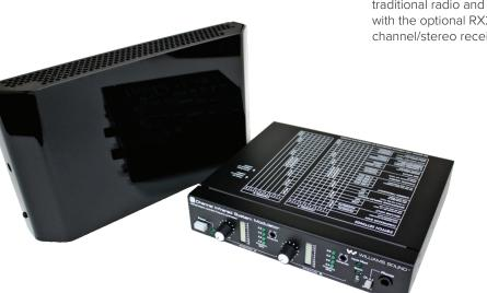
The WIR TX925 is ideal for simultaneous language interpretation for up to two languages. It can operate up to 19,000 sq ft in two channel mode or up to 30,000 in single channel mode. Operating on 2.3 and 2.8 MHz, the WIR TX925 is less susceptible to traditional radio and lighting interference. Listen to the program with the optional RX22-4 four-channel receiver or the RX18 twochannel/stereo receiver.
