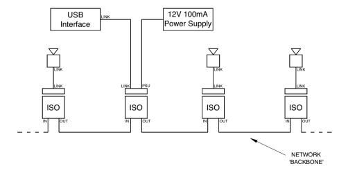
6. Both Tannoy's SENTINEL and Ethernet interface can provide sufficient power for one ISOLATOR
