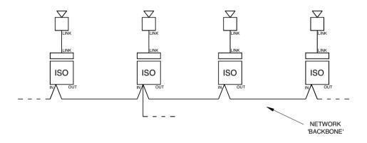
3. ISOLATORs may be used to segment a large network as convenient, protecting each segment from the others. Note that using them in this way does NOT allow the network to exceed the 1km total maximum length limit
