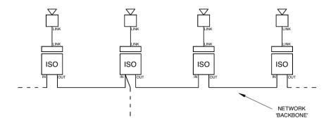
2. Using only the Phoenix IN (or OUT) ports allows the network wiring to be installed and tested before other equipment is installed
