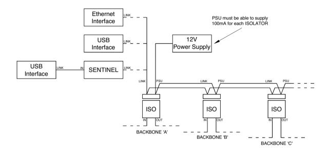
5. Because of the limited power available from a USB interface, connecting Linea's USB interface directly to an ISOLATOR will not work unless an external power supply is connected either to the rear of the USB interface or, as shown, to the ISOLATOR
