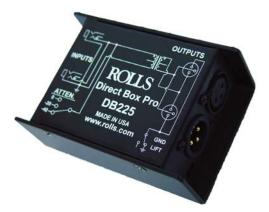
A passive direct box designed to take high impedance signals and convert them to low impedance. The unit features an attenuator switch for padding the input signal by either 20 or 40dB, and a ground lift switch that may be used to reduce unwanted hum caused by ground loops. All in a very heavy metal chassis MADE IN THE USA.
