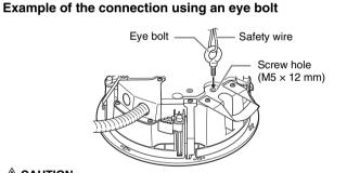
**⚠** CAUTION Always take measures to prevent the speaker from falling down. Use a safety wire of appropriate length. Should the speaker fall and the wire is too long, the wire may snap due to excess strain.
