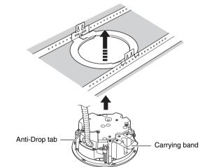
Make sure the release lever is in the position of the figure below. If it is set to the position of the figure, when all the Anti-Drop tabs cross over the O-ring, the speaker is held temporarily.
