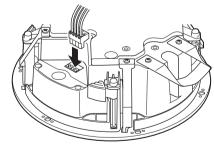
5 Tighten the screw and then attach the terminal cover.
