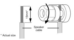
Be sure that the bare wire ends do not jut out from the terminals and touch the chassis.
