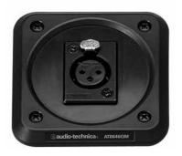
shock isolator designed to minimize the pickup of mechanical noise from the mounting surface. The associated microphone shall plug into the mounting plate via a 3-pin XLRF-type input connector and a 3-pin terminal strip shall be provided on the bottom of the plate for audio output. The unit shall offer a low-reflectance black finish. The unit's dimensions shall be: 78.0 mm (3.07") wide, 78.0 mm (3.07") deep, 8.4 mm (0.33") high. Weight of the shock mount less microphone, shall be 64 g (2.3 oz).
