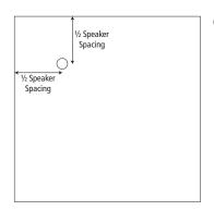
C. Place the first loudspeaker at ½ the Loudspeaker Spacing distance from any corner of the room.
