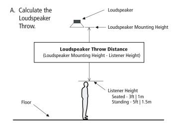
B. Calculate the Loudspeaker Spacing distance by multiplying the Loudspeaker Throw Distance by the Coverage Multiplier.
