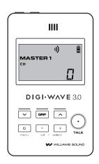
Must be set to 1-way Repeater mode, MASTER, GROUP 0-1023. The unit will default to CH 0. NOTE: For more than one repeater, repeaters on additional channels must be GUEST.
