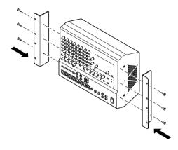
**3.** Carefully store the remaining six screws that are not used in Step 2 so they are not lost. Once the rack-mount brackets are installed there will be a total of eight empty screw holes on the both sides of the mixer.
