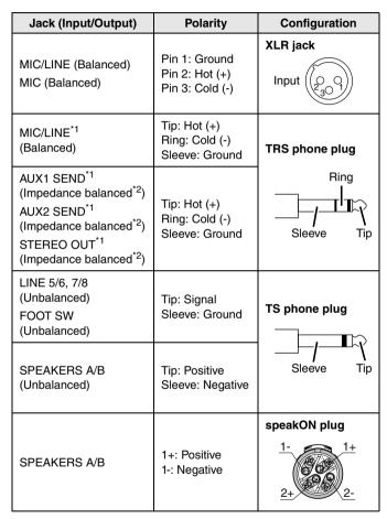
\*1 These jacks also can be connected with TS phone plugs. If you use TS phone plugs, the connection will be unbalanced.
