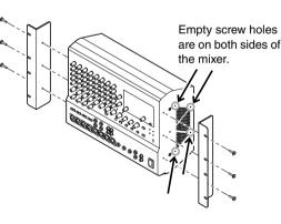
**4.** If you wish to remove the rack-mount brackets and reinstall the side pads, ensure that they are installed on the correct sides of the mixer. The inside surface of the side pads are marked as "L" (Left) or "R" (Right).
