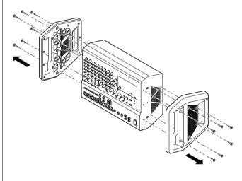
**2.** Use six of the screws you removed in Step 1 to securely install the RK-EMX7 separately sold (rack-mount brackets) onto the mixer.
