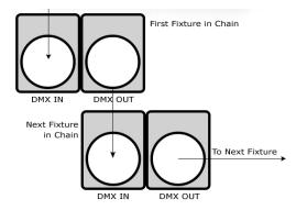
A quick note: Often, the setup for Master-Slave and Standalone operation requires that the first fixture in the chain be initialized for this purpose via either settings in the control panel or DIP-switches. Secondarily, the fixtures that follow may also require a slave setting.
