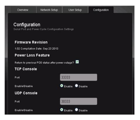
To connect to IP15 over TCP, simply start your TCP client program ( such as Hercules or PuTTY) and specify the IP address of the iP15 and the TCP port. Start the connection ( many programs have a Connect button to start the connection ) and type iP15 console commands such as Help. You should see the reply to the command on the TCP client terminal window. See page 13 and 14 of this manual for a full list of the console commands available.
