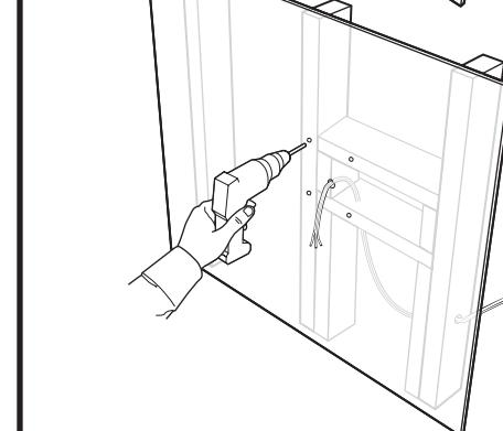
Minimum Installation Requirements when mounted to wood studs:  $\frac{1}{4}'' \times 1\frac{1}{2}''$  (M6 x 38 mm) lag screw
