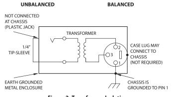
Figure 2. Transformer Isolation
