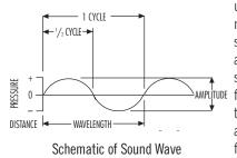
usually produces many frequencies simultaneously. In any such complex sound, the lowest frequency is called the fundamental and is responsible for the pitch of the sound. The higher
