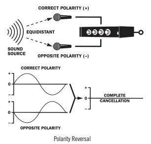
Although there is an international standard for microphone polarity (pin 2+, pin 3-), a reversal may be found in an incorrectly wired microphone cable. It can be identified by checking each microphone and cable against a microphone and cable that are known to be correct. In any installation, all microphones and microphone cables must have the same polarity.
