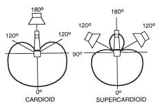
Monitor Speaker Placement For Maximum Rejection: Cardioid and Supercardioid
