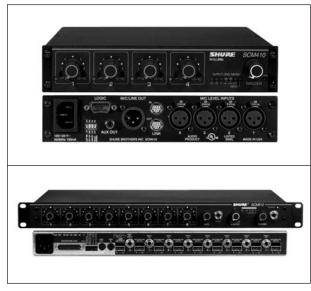
Examples of Automatic Microphone Mixers (shown front and back)
