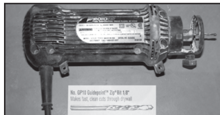
Fig. 11: Rotozip™ showing guidepoint bit.
