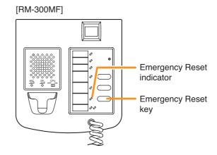
Input a reset signal to the Emergency Control Input terminal of the VM-3240VA, VM-3360VA, VM-3240VA, or VM-3360E which has been assigned a reset function.
