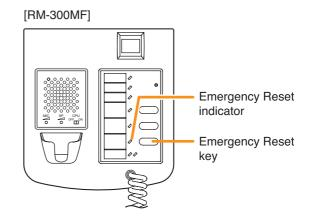
Input a reset signal to the Emergency Control Input terminals of the VM-3240VA, VM-3360VA, VM-3240E, or VM-3360E which has been assigned a reset function.
