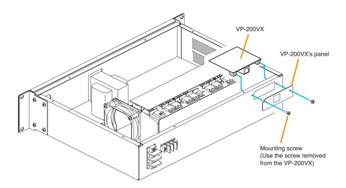
Step 4. Plug the VP-200VX's connector into the CN106 connector on the circuit board inside the amplifier.
