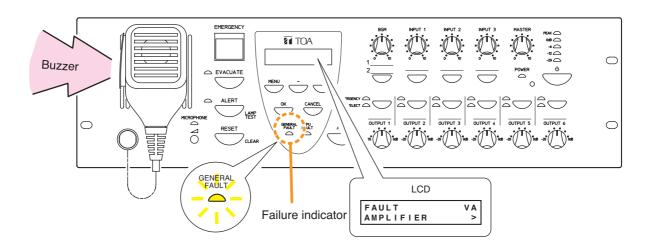
In this event, a failure of the contents shown on the LCD screen has occurred within the system. Pressing the amplifier's [OK] key to acknowledge the failure or acknowledging the failure by way of the Fireman's Microphone stops the buzzer and switches the yellow failure indicator from flashing to steady-on mode. (Refer to "Failure Acknowledgement" on page 54).
