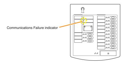
A failure has occurred in communications between the RM-200M and the VM-3240VA or VM-3360VA. The previous status is automatically restored if communications return to normal.
