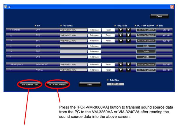
Press the [VM-3000VA->PC] button to transmit sound source data from the VM-3360VA or VM-3240VA to the PC. Sound source data written into the VM-3360VA or VM-3240VA is read into the current registration screen.
