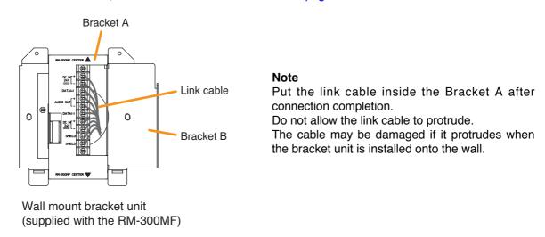
Step 3. Plug the RM-300MF's connection cable into the connector port on the wall mount bracket unit.
