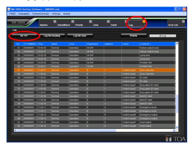
Pressing the [VA  $\Rightarrow$  PC] button starts the transmission of log data from the VM-3360VA or VM-3240VA to the PC.
