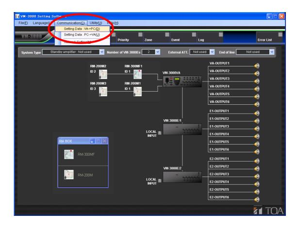
Selecting "Setting Data: VA->PC" allows PC-set data written to the VM-3360VA or VM-3240VA to be read into the software.
