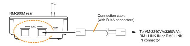
• The following table shows the maximum cable distance when STP Category 5 straight cable (with RJ45 connectors) is used.
