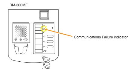
A failure has occurred in communications between the RM-300MF and the VM-3240VA or VM-3360VA. The previous status is automatically restored if communications return to normal.
