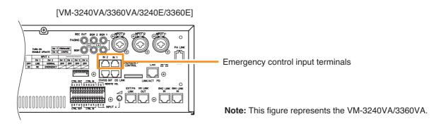
**Step 2.** The Alert or Evacuation announcement is broadcast over the zone(s) assigned to the Emergency Control Input terminals. The Emergency indicator flashes red, the buzzer sounds and the Alert or Evacuation Announcement indicator lights red. At the same time, the Output indicator corresponding to the set broadcast zone(s) lights.
