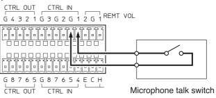
The corresponding all-zone call or output indicator lights green, allowing microphone announcements to be broadcast from the corresponding speaker line.
