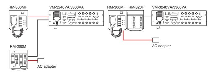
• By supplying power to the RM-300MF/320F from the VX-2000DS, the RM-300MF/320F can be operated on the backup power even in case of AC power failure.
