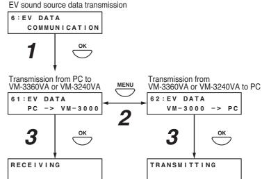
**Step 4.** Activate the setting software to transmit the EV sound source data from the VM-3360VA or VM-3240VA, then click "Utility->EV" on the menu bar.
