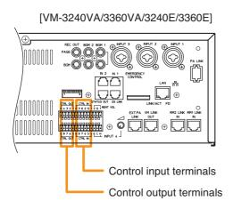
[Example] Connecting a timer to Control Input Terminal 1
