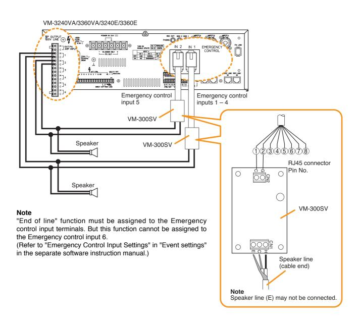
**Tip**Use a cable fitted with RJ45 connectors for connection to the Emergency control input terminal.
