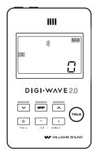
Must be set to Repeater, CH 0 and MAS. NOTE: For more than one repeater, repeaters on additional channels must be SLV.
