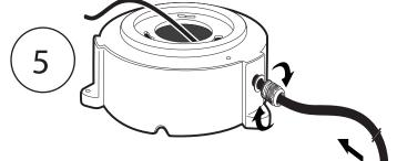
Install the gland nut into the hole as shown above in #6 and feed external wire from outside through the gland nut and up through the center hole in the lower half of the speaker as shown above.
