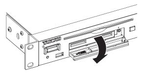
2. Inserted SD cards with the correct orientation. The label should be up and the connector should be inserted toward the back.
