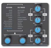
Signature 16 has a single internal Lexicon FX processor and send/return bus for adding FX such as reverb, delay, Chorus, Rotary, LoFi, Tape emulation, and more. Signature 22 and 22MTK have dual processors and send/return paths. Each Effect has two adjustable parameters. Refer to section 8.0 for more detail.
