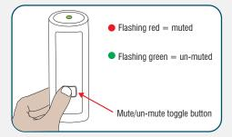
To turn microphones off, first mute the microphone, and then plug **Sten #4** it into the Charger Base. Make sure the RED LED turns on. Optionally, the microphone can be turned off manually. Simply press and hold the MUTE button for  $\sim$ 10 seconds until the LED turns solid RED and release button.
